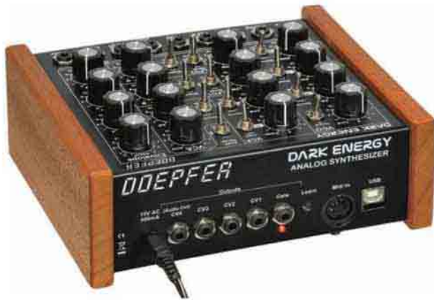
Fig. 1. Four CV outs translate MIDI note info, pitch-bend, velocity, and one CC (assigned via the Learn button) into the analog world. That the MIDI info can come in from the USB port makes the Dark Energy a useful computer-to-analog-synth interface as well as a synth in its own right.
