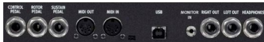
Fig. 2. The rear panel includes a 1/8" input for an MP3 player, routed to the headphone output for when you're learning tunes. At your option, the Electro 3 can send organ to the left main output and non-organ sounds to the right, so you can use a real rotary speaker on organ while everything else goes straight to your mixer.
