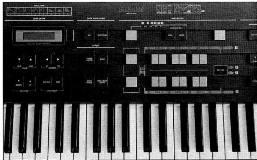
Closeup of the voice programming section of the CZ-5000, which is electronically identical to that on the CZ-101.
