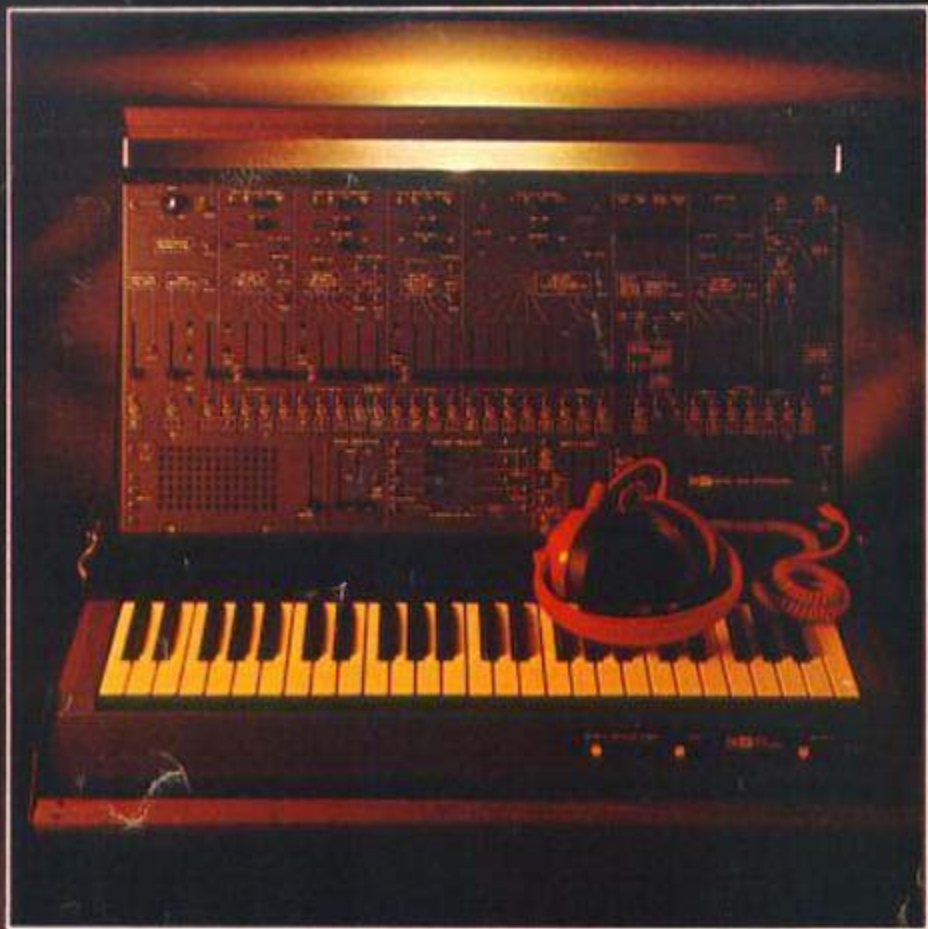
Above: Suitcase-size portable synthesizer not only realistically imitates organs, electric pianos and other conventional instruments but also permits the performer to invent his own out of the unit's wide range of sound, by ARP Instruments, $2795.
