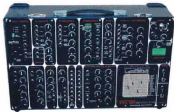
FIG. 1: Bearing some physical resemblance to the vintage EMS Synthi A, the Analogue Solutions Vostok is a complete modular synthesizer in a suitcase.
