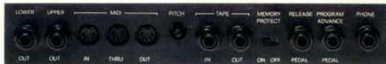
The back panel from left to right: Audio Outputs (Lower/Upper) MIDI (IN-THRU-OUT) - PITCH (General) - TAPE (IN/OUT) - MEMORY Protect switch (IN/OUT) - RELEASE Pedal - PROG. ADVANCE Pedal - PHONE Input.
