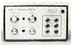
The 73-B has improved immunity to harmonics, and can produce an accurate output within two cycles of when input is applied. The output is an adjustable 1-volt/octave control voltage, with trigger provided for different makes of synthesizers. Freedom from keyboards at last.
